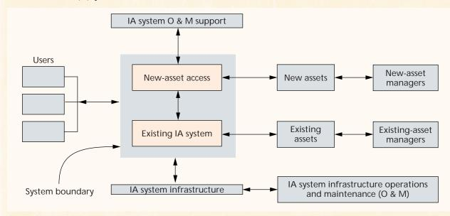
The system boundary focuses on the automated applications portion of the operation and defines such external entities as users, operators, maintainers, assets, and infrastructure (campus networks, etc.) as part of the system environment. The diagram abstracts out such additional needed capabilities as asset catalogs and direct user access to O&M support and asset managers. Some stakeholder roles and responsibilities include:
